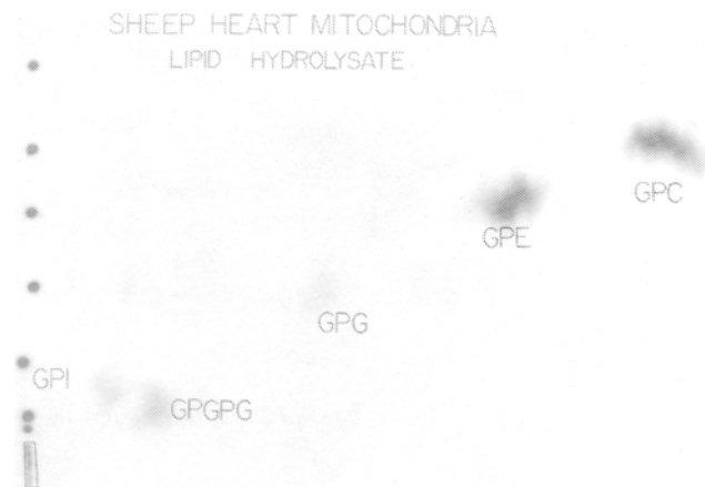
FIG. 7. Radioautograph of neutron-activated chromatogram of deacylated sheep heart mitochondrial lipids. Note 1\ \mu\text{g} phosphorus samples applied near edges of developed chromatogram.
